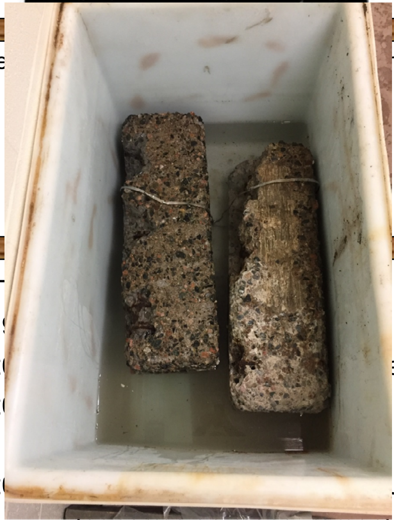
for corrosion measurements
